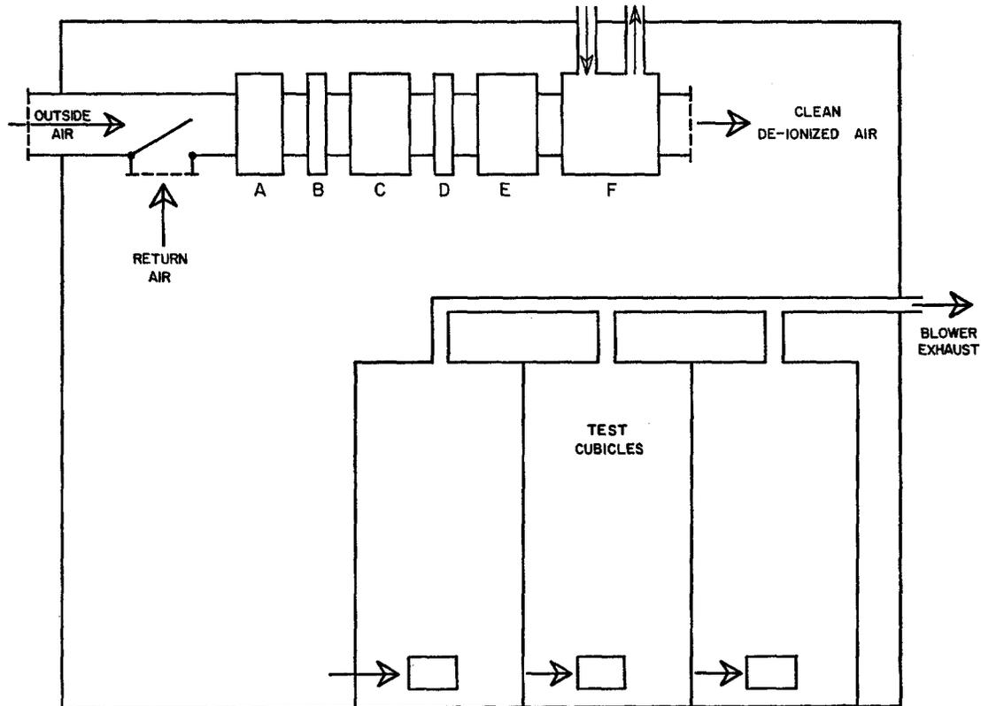
FIGURE 2. Diagram of air purification unit designed to provide clean air for gaseous ion investigations. *A*, electric duct heater. *B*, prefilter for *C*. *C*, electrostatic precipitator. *D*, negative ion source to neutralize excess positive ions generated in *C*. *E*, activated carbon filter. *F*, air conditioner.
